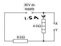
The power transferred in the  $4.0\,\Omega$  heater is  $9.0\,W$ .
