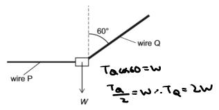
The radius of wire Q is twice the radius of wire P.
