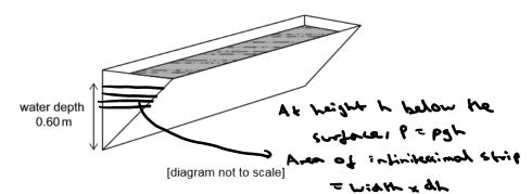
The trough contains water of depth 0.60 m measured on the vertical rectangular face.
