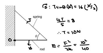
The spring constant of the spring is  $20\,\mathrm{N\,m^{-1}}$  and the weight of the rod is  $16\,\mathrm{N}$ .
