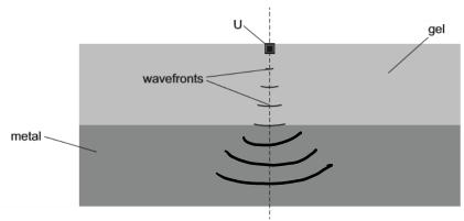
Ultrasound travels faster in the metal than in the gel.
